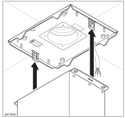
■ Using at least two people, lift the hood and guide the spring clips through their respective slots in the flange at the top of the chimney.
